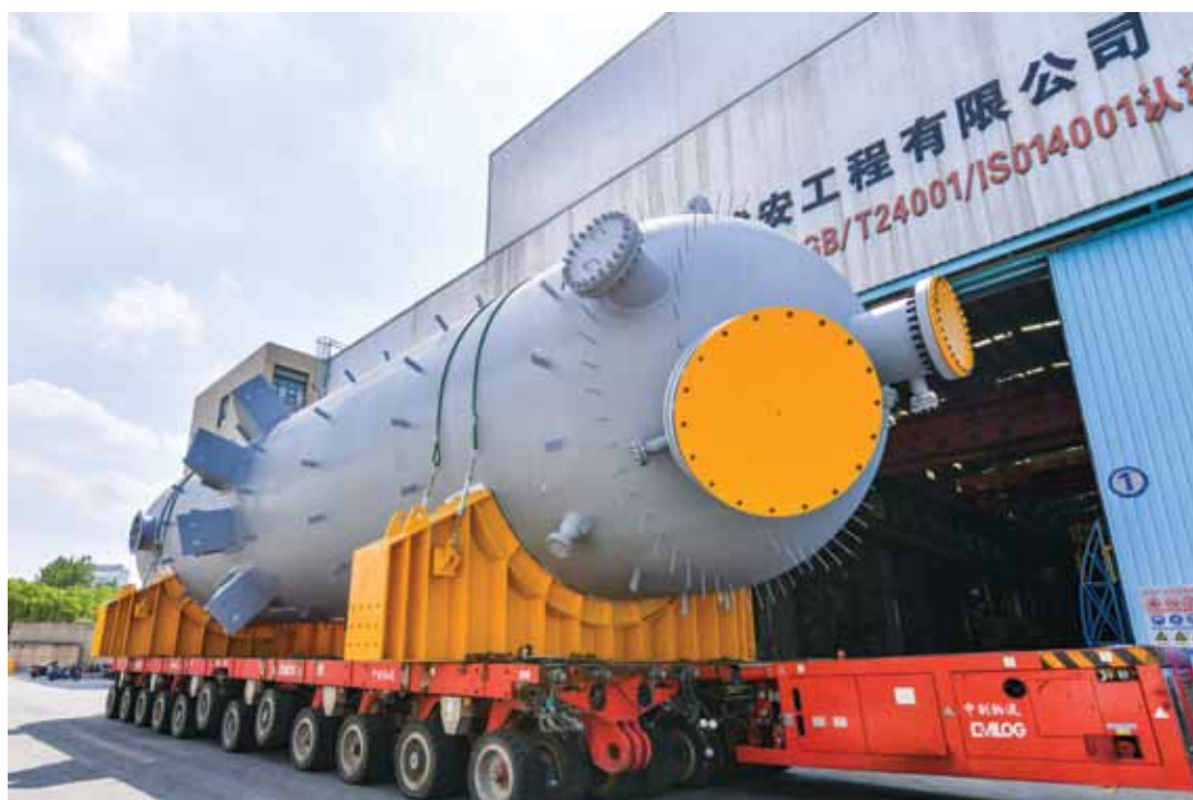
➤ Spiral tube heat exchanger ready for delivery
